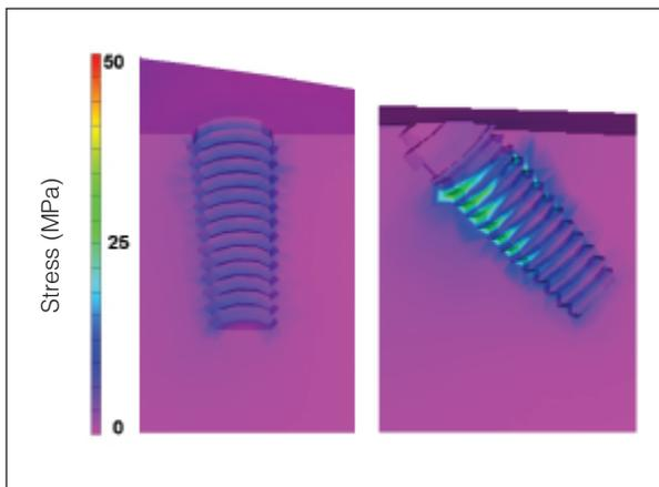
**Fig 3** Von Mises stresses (MPa) around single implants submitted to a vertical load of 150 N in cortical bone. (left) The 0-degree model (max stress: 10.6 MPa). (right) The 45-degree tilted model (max stress: 25 MPa).
