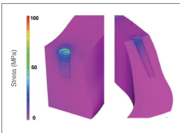
**Fig 5** Von Mises stresses (MPa) around splinted distal implants submitted to a vertical load of 150 N in cortical bone. Details are shown without framework visualization. (left) The 0-degree model with cantilever extensions of 15 mm (max stress: 75 MPa). (right) The 45-degree tilted model with cantilever extensions of 5 mm (max stress: 25 MPa).
