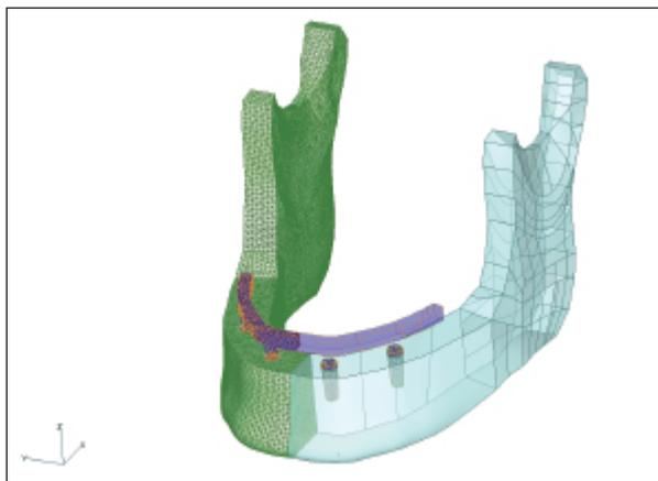
**Fig 2** Edentulous jaw 3D model. Four parallel wall screw-type implants were placed in the interforaminal area of the mandible, simulating the clinical treatment of an edentulous patient with an FFP. The first analyzed configuration had vertical bilateral distal implants and cantilevers of 15 mm.
