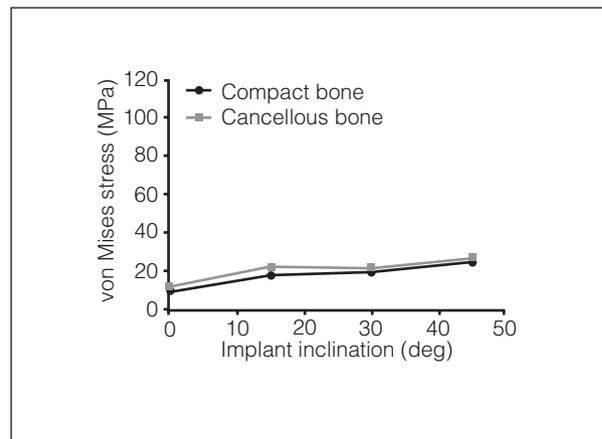
**Fig 4** Test 1 results. Stress values (in MPa) in the single implant model submitted to a vertical load of 150 N.
