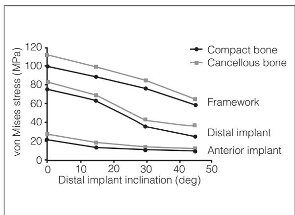
**Fig 6** Graphic representation of stress reduction observed in the peri-implant bone surrounding distal and anterior implants splinted in a rigid FFP submitted to a vertical load of 150 N. Implant inclinations, cantilever lengths, and cancellous/compact bone values are plotted. Metal framework stresses have also been plotted.
