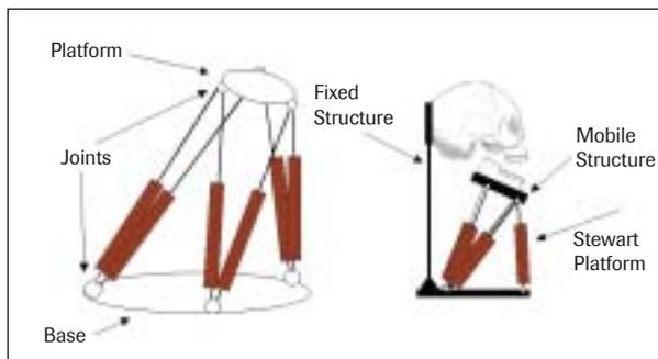
**Fig 1** Schematic diagram of the masticatory robot.
