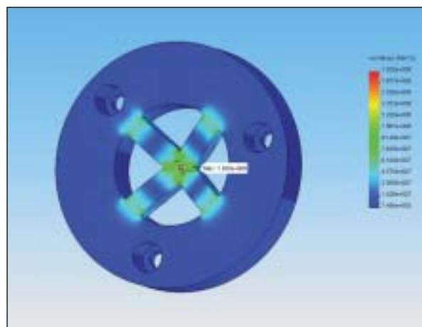
**Fig 6** COSMOSXpress simulation of the behavior of the sensor-equipped base when loaded. The application of a force of 80 kg along the vertical z-axis was simulated to show the resulting deformation. The illustration highlights the zones of maximum stress on the structure and verifies that the model can support the maximum load.
