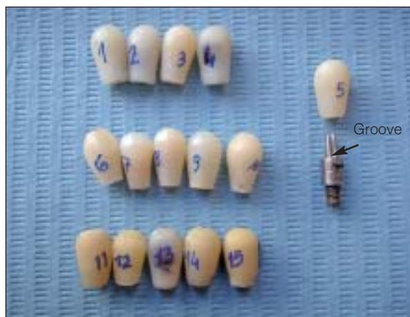
**Figs 12a and 12b** Each sample produced was measured on its main and smaller axes with a caliper to verify that all the crowns were identical.
