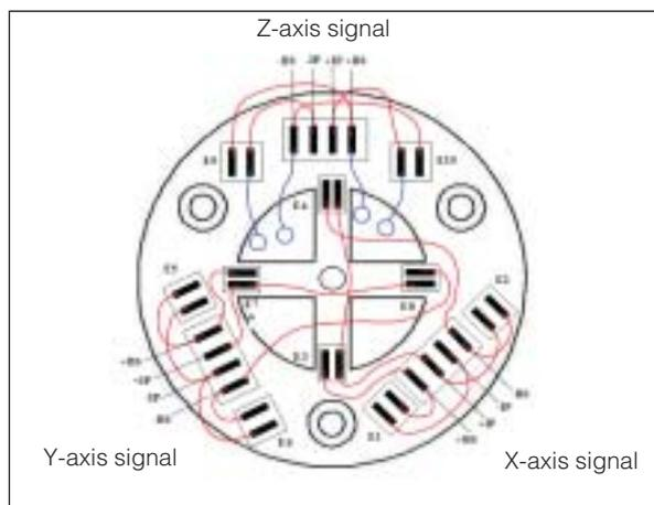
**Fig 4** Upper face of the sensor-equipped base showing the wiring. Red line = Upper face connecting wires; Blue line = Wires connecting upper and lower faces; Dotted line = Wires connecting the sensor to the amplifier; +BS/-BS = Power supply to the bridge; +IP/-IP = Bridge output.
